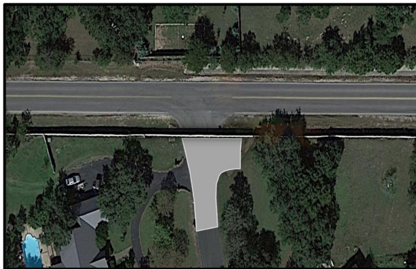
Figure 22 – Partial Hammerhead Turnaround
