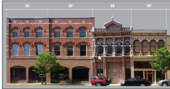
Figure 7-3 Illustration showing building articulation requirement
