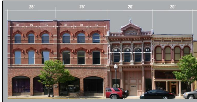
Figure 7-3 Illustration showing building articulation requirement
