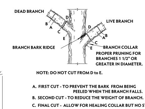
PEELED WHEN THE BRANCH FALLS. B. SECOND CUT - TO REDUCE THE WEIGHT OF BRANCH. C. FINAL CUT - ALLOW FOR HEALING COLLAR BUT NO STUBS **LEGEND**
