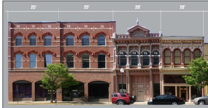
Figure 7-3 Illustration showing building articulation requirement
