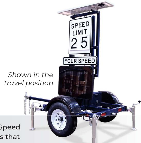
Easy to tow and quick to set up, the Stalker Street Dynamics Speed Alert Monitor 3 (SAM 3) features 18-inch amber LED characters that are visible at up to 1000 feet. A convenient hand-held controller, K-Band Doppler radar, and an 8-10 day battery with solar panel round out its standard configuration.
