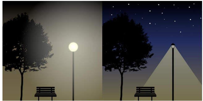
Shielded lights help to reduce light pollution by directing light only to the area intended.
