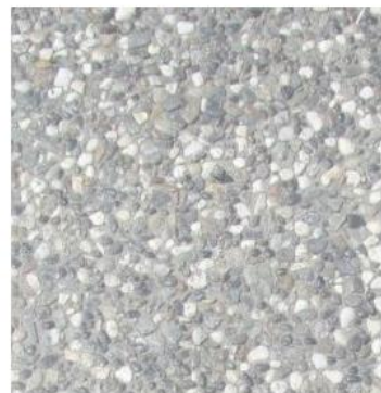
Concrete Flatwork heavy aggregate finish
