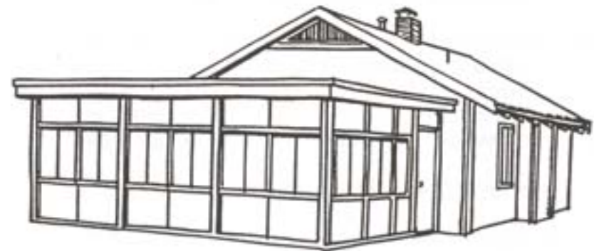
Addition is not acceptable with existing building's architectural style
