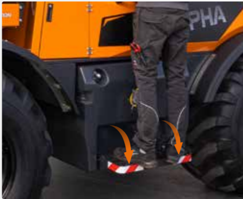
Retractable folding step for easily access at maintenance
