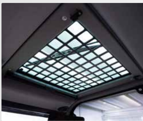
Roof window with safety grill, sunshade and windshield wiper
