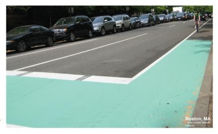
• When the dominant motor vehicle traffic flows right and bicycle traffic continues through (such as a Y intersection or access ramp).
