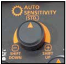
Auto Mode sensitivity adjustment dial
