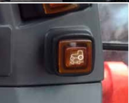
Xpress Restart Allows the operator to directly control the main clutch by simply pressing the brake pedals. The tractor can be stopped without using the clutch pedal, helping to ensure maximum convenience and productivity.
