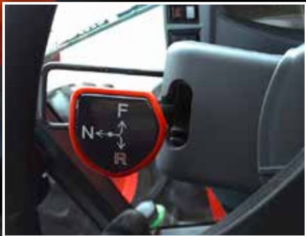
Momentary Shuttle Lever Located behind the steering wheel, the one touch momentary type shuttle lever allows easy shifting between forward and reverse while keeping both hands on the wheel.
