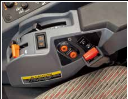
Operating Levers with Armrest Operating levers and switches for controlling hydraulics and shifts offer an ergonomically-designed armrest to increase ease of use and reduce fatigue.
