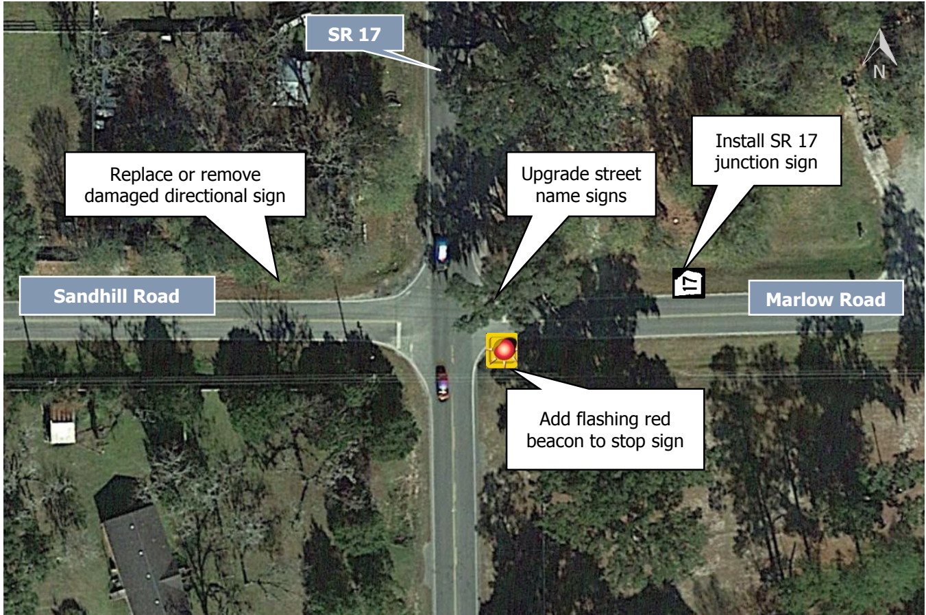
FIGURE 4-12. RECOMMENDED SHORT TERM SIGNAGE IMPROVEMENTS
