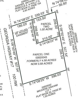
IRF-5/8" REBAR FOUND IRS-1/2" REBAR SET STK-WOODEN STAKE FOUND ERROR OF CLOSURE: EXCEEDS 1':10,000' PLAT NOT ADJUSTED
