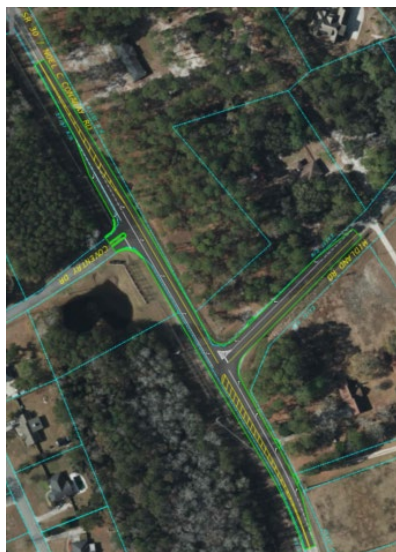
Figure 2-Left Turn Lanes-Secondary Alternative
