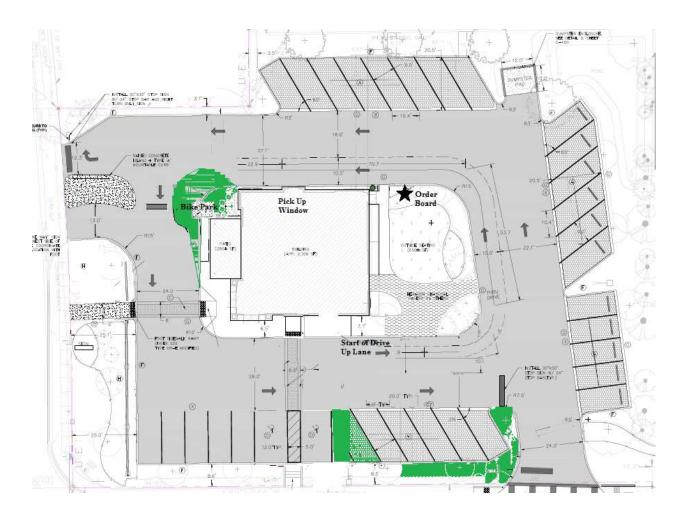
In addition, an increase in queue length is recommended by moving the order/menu board five feet east of the sidewalk from the outdoor patio to the north parking area. Staff recommends provision of a cross walk and adding pavement striping to delineate the drive through lane staff recommends approval. This will help to serve the health, safety and welfare of the city.
