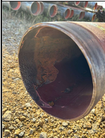
5. Column Pipe - Interior Pitting
