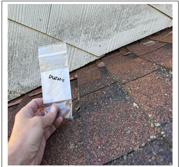
Sample D92525-11: Tar on roof negative for asbestos.
