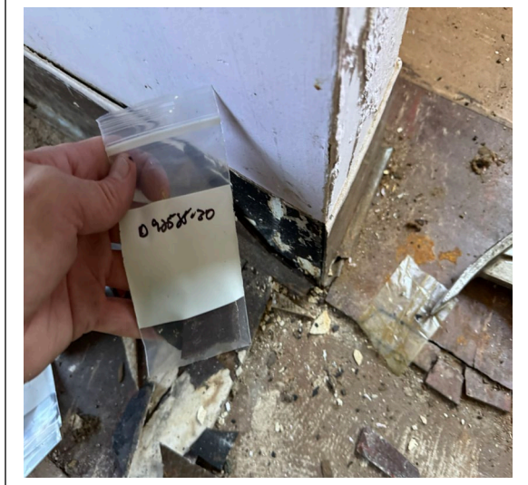
Sample D92525-30: Base cove/adhesive end floor bedroom negative for asbestos.
