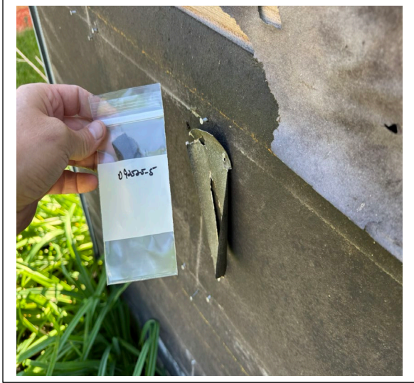
Sample D92525-5: Tar strips behind siding negative for asbestos.
