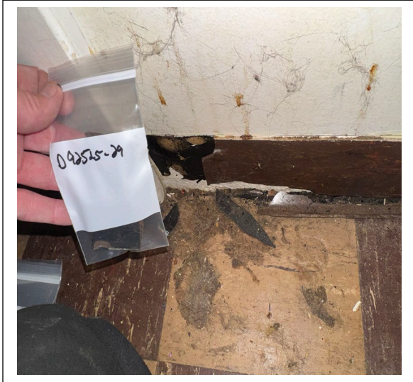
Sample D92525-29: Base cove/adhesive end floor bedroom negative for asbestos.
