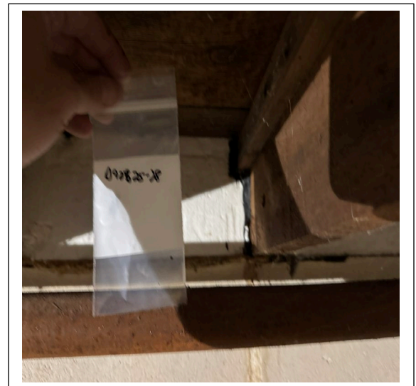
Sample D92525-28: Black caulking in the basement, rim joist, positive for asbestos.
