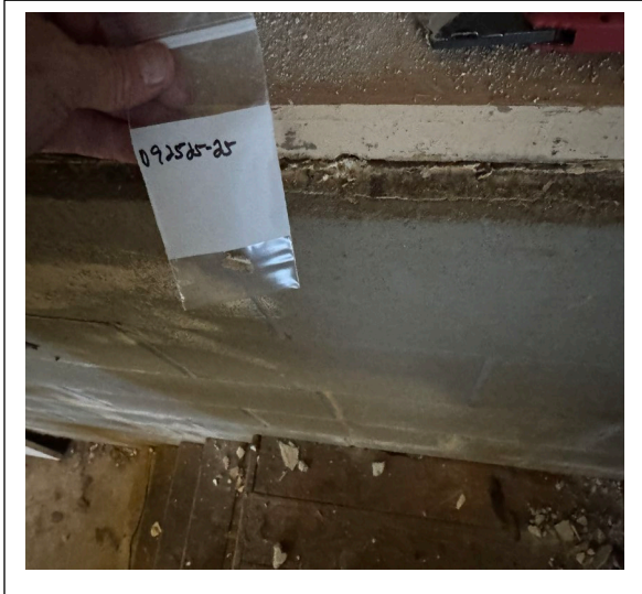
Sample D92525-25: Caulking, White, at rim joist in basement negative for asbestos.
