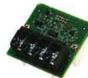
Fig. 12: Load Current Card (Accessory 23GA/GB)
