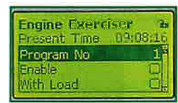
Fig. 13: Programmable Engine Exerciser
