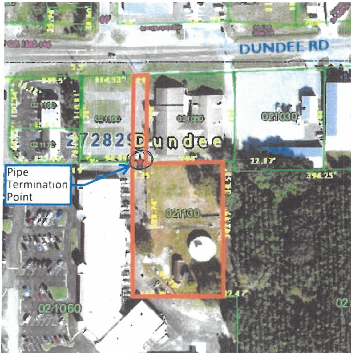
Figure 1. 14-inch Pipe Termination Point at Dundee WTP
