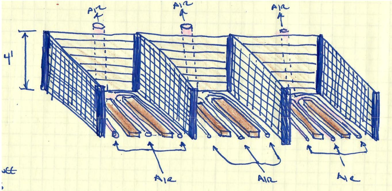
Railroad ties will be used as protective guides for the tractor bucket to slide on so that the piping isn't damaged.
