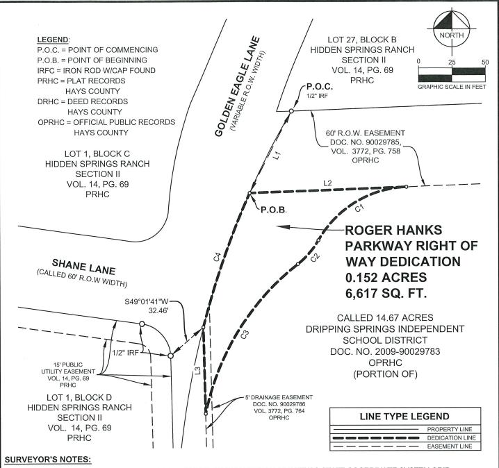
THE BEARINGS, DISTANCES, AREAS AND COORDINATES SHOWN HEREON ARE TEXAS STATE COORDINATE SYSTEM GRID, CENTRAL ZONE (FIPS 4203) (NAD'83), AS DETERMINED BY THE GLOBAL POSITIONING SYSTEM (GPS). THE UNIT OF LINEAR MEASUREMENT IS U.S. SURVEY FEET. A METES & BOUNDS DESCRIPTION AND A LINE & CURVE TABLE WERE CREATED IN CONJUNCTION WITH THIS RIGHT-OF-WAY DEDICATION BOUNDARY EXHIBIT.
