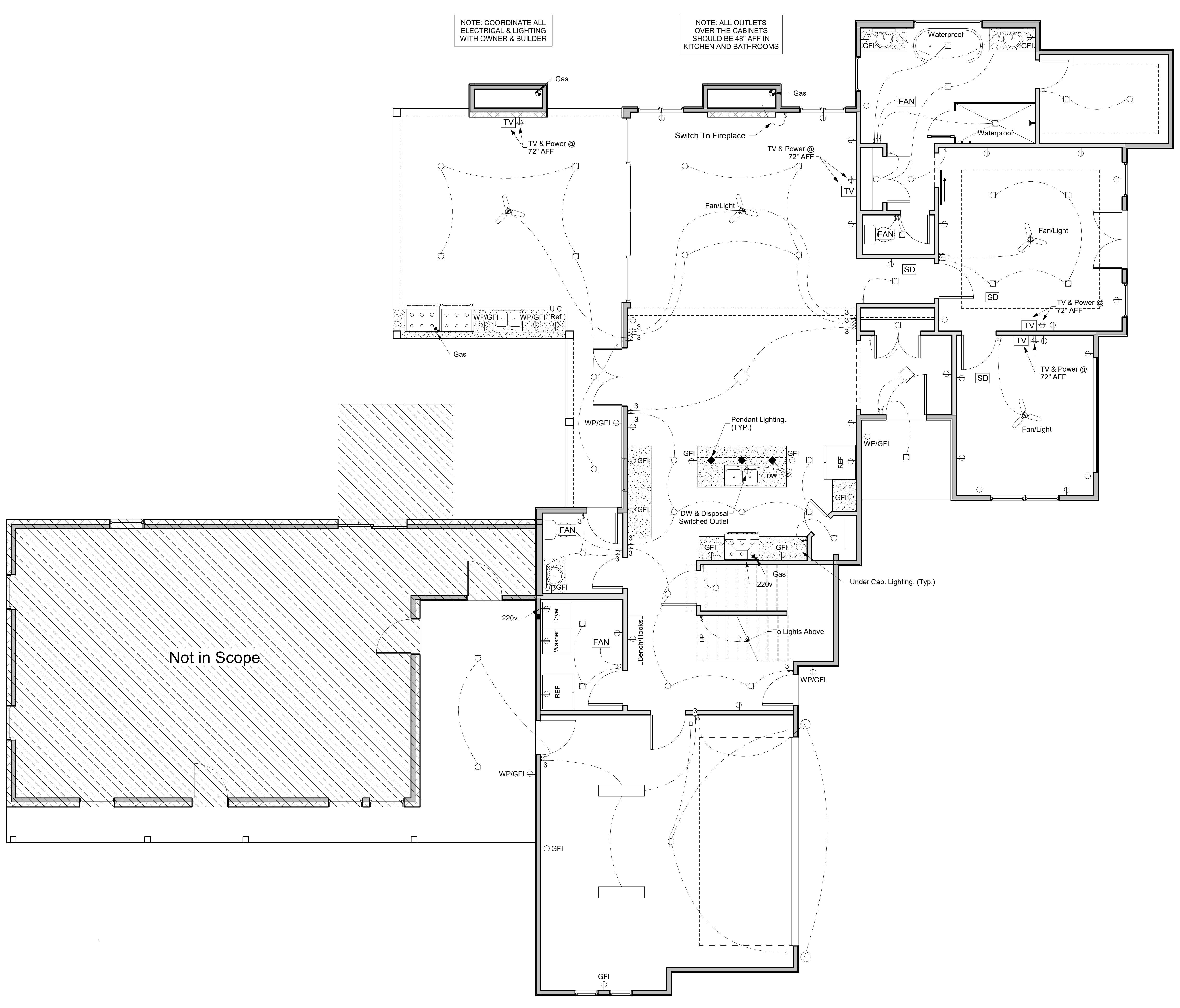
1 Level 1 - Remodel Electrical Plan 1/4" = 1'-0"
