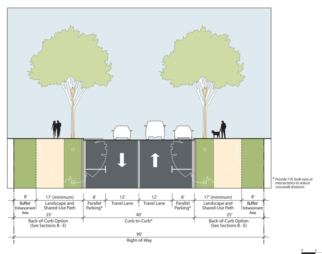
2 Lane Commercial Collector with Parallel Parking City of Dripping Springs - Transportation Master Plan
