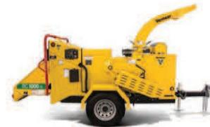
**CLUTCHLESS PTO.** The throttle integrated with the belt drive engagement process helps ensure that the PTO can only be engaged while the engine is at low idle/low rpm. Automatically, the engine throttles up to full rpm after the belt drive is fully engaged. This system helps to reduce premature wear to the belt drive system by preventing high idle engagement of the cutter drum.
