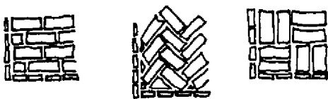
Brick Paving Patterns
