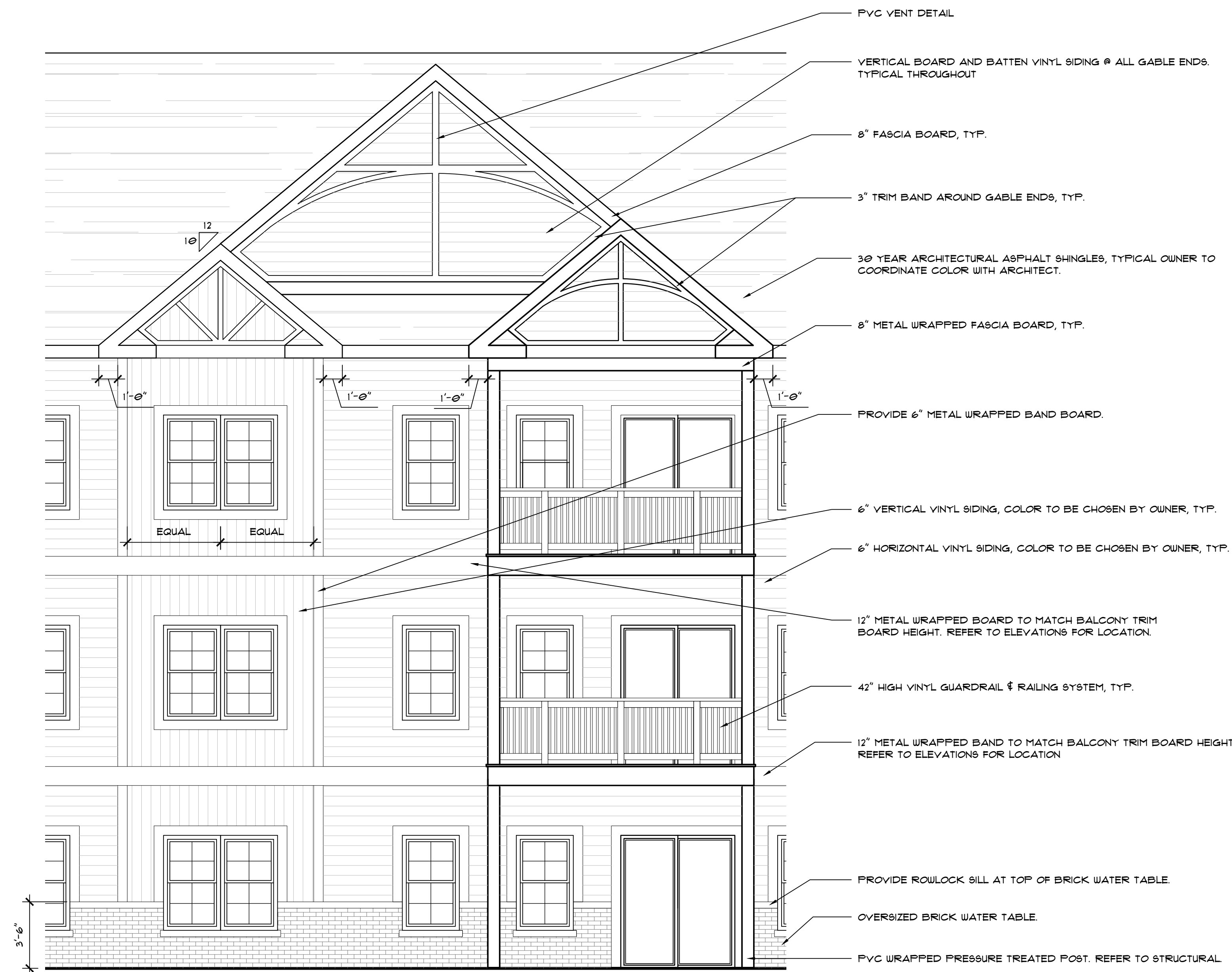
1 ELEVATION DETAIL: REAR GABLE GROUP SCALE: 1/4" = 1'-0"
