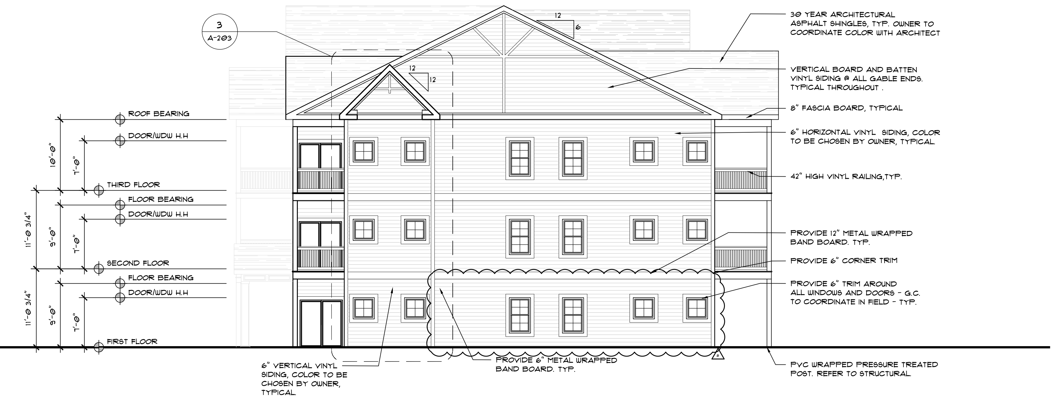
24 UNIT BUILDING: RIGHT ELEVATION SCALE: 1/8" = 1'-0"
