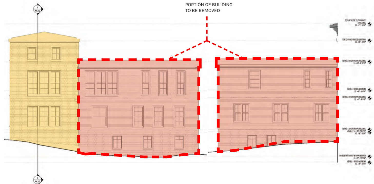
21 The Green - East Elevation
