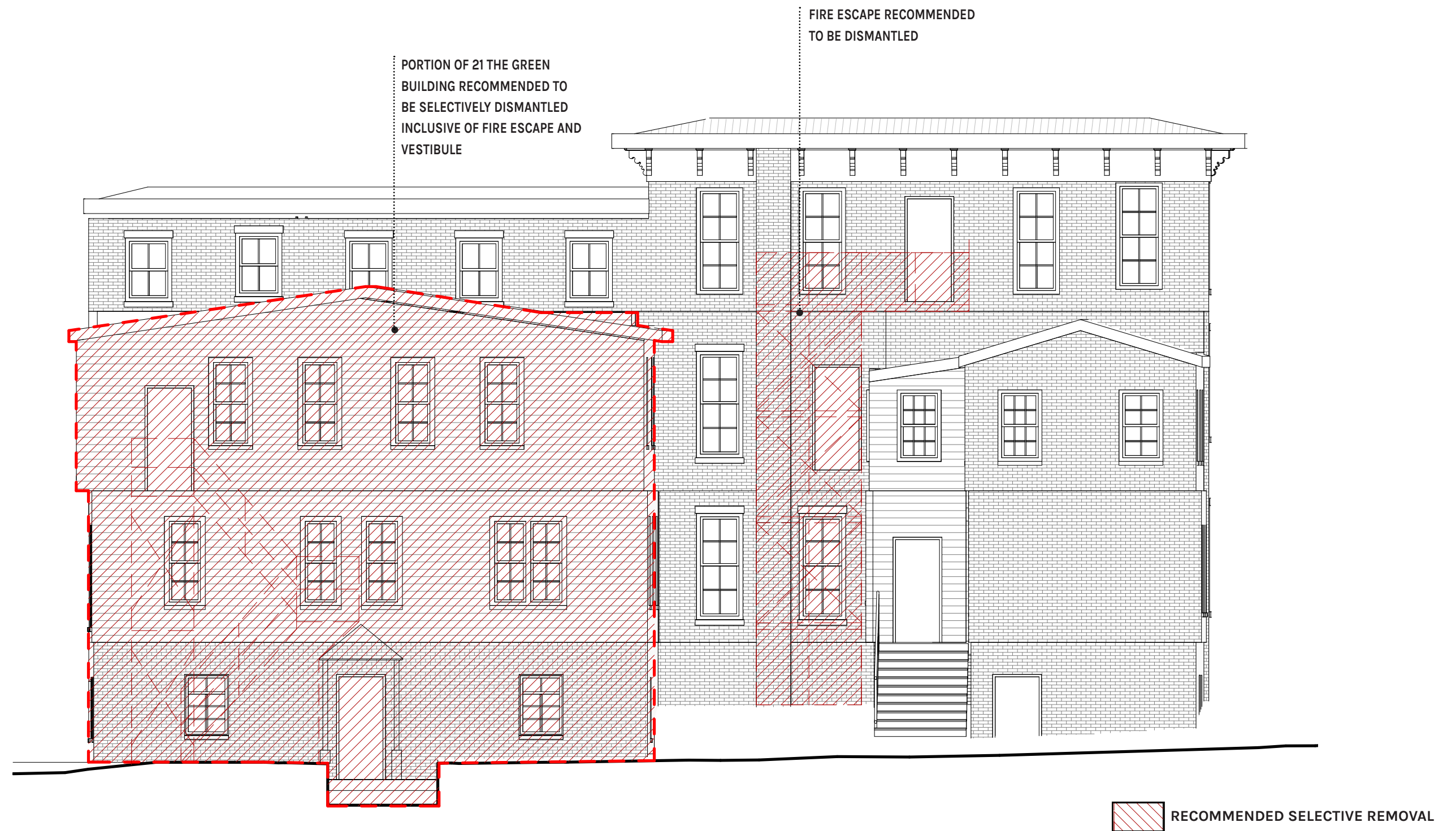
Figure 4.2.6 15 and 21 The Green Rear Elevation - Selective Removal
