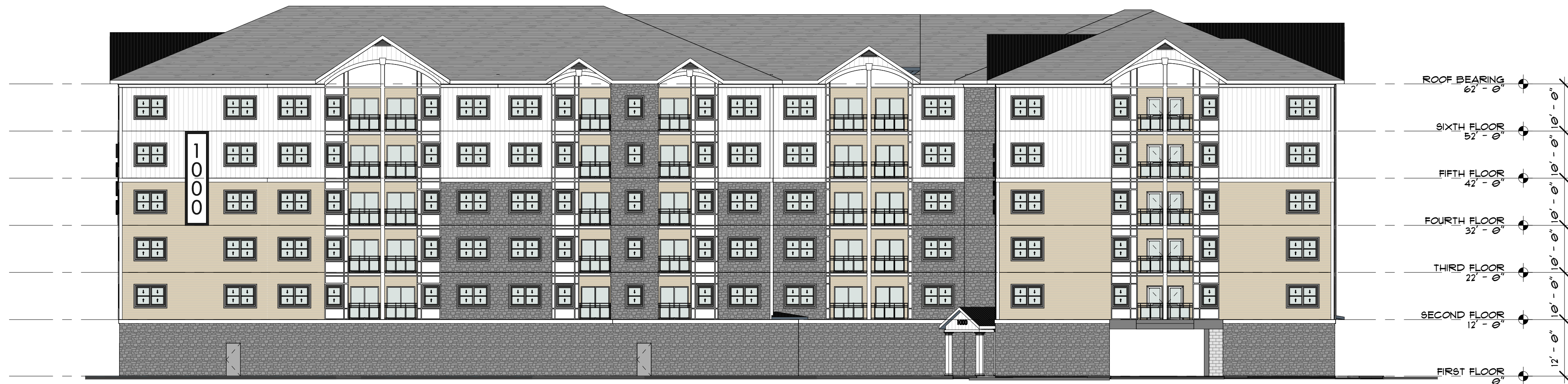
② SOUTH ELEVATION - BUILDING 2 1/16" = 1'-0"
