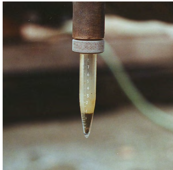
Figure 2-4: Rossum Sand Tester on Development Discharge Line – Stantec will closely monitor develop progress to track well performance and sand production.
