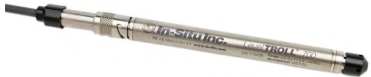
Figure 2-1: Example Level Transducer used for Zonal Falling Head Testing
