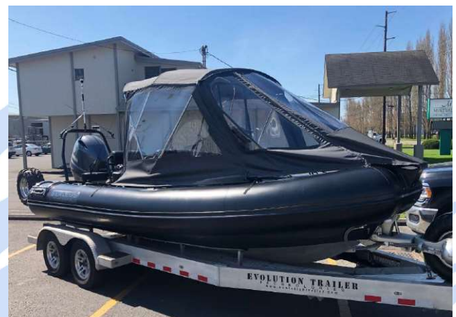
Figure 3 The 20' "SeaLegs" skiff, launched and recovered from the Q105, to be used for shallow water survey.
