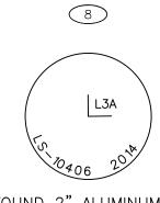
FOUND 2" ALUMINUM CAP FOUND 2" ALUMINUM CAP ON 5/8" REBAR AT GRADE GOOD CONDITION
