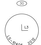
FOUND 2" ALUMINUM CAP FOUND 2" ALUMINUM CAP FOUND 2" ALUMINUM CAP ON 5/8" REBAR ON 5/8" REBAR ON 5/8" REBAR AT GRADE 0.2' ABOVE GRADE 0.5' ABOVE GRADE GOOD CONDITION GOOD CONDITION GOOD CONDITION -HELD-
