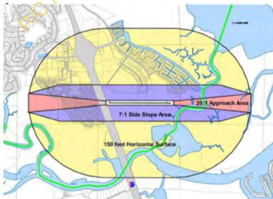
Figure 2.1 - Airport Height Restrictions
