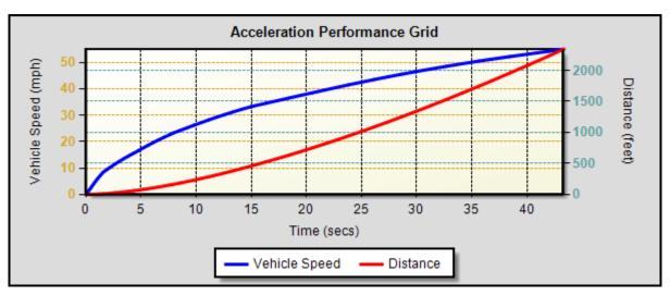
Acceleration Performance: TIME TO ACCELERATE ON A GRADE TO 55.0 (MPH) IS 43.35 (SECS)
