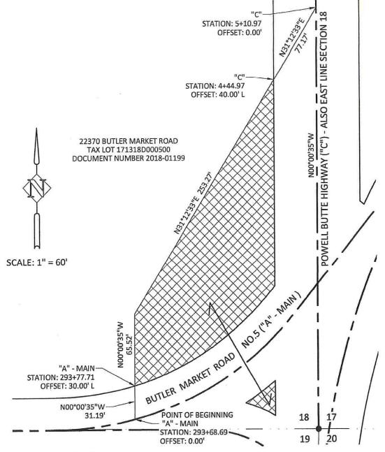
BEARINGS AND ROAD STATIONING ARE PER CS21027 DESCHUTES COUNTY SURVEY RECORDS.
