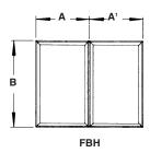
Dampers larger than maximum single section are an assembly of equal size single section dampers (maximum section size 48"w x 72"h (1219 x 1829) and may be coupled for operation in a variety of ways. A 1" (25) diameter jackshaft is normally used for multiple section coupling.
