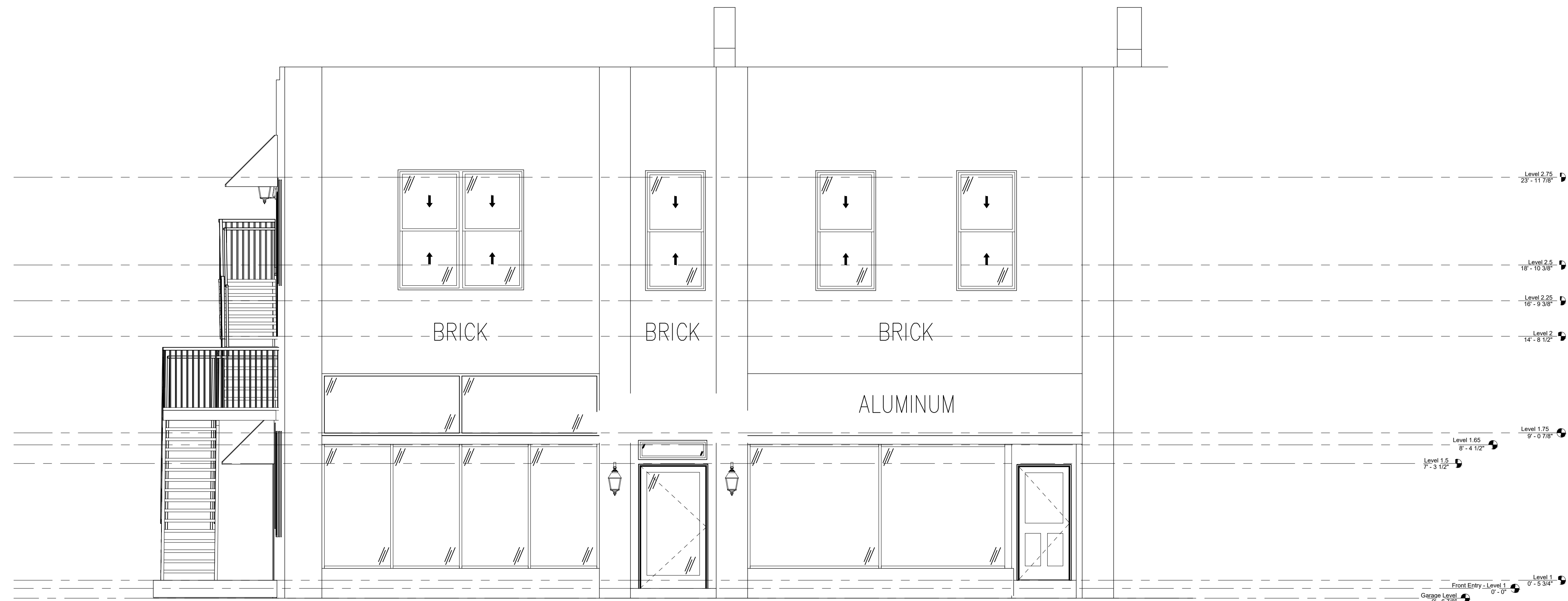
1 FRONT ELEVATION A3.0 SCALE: 1/4"=1'-0"
