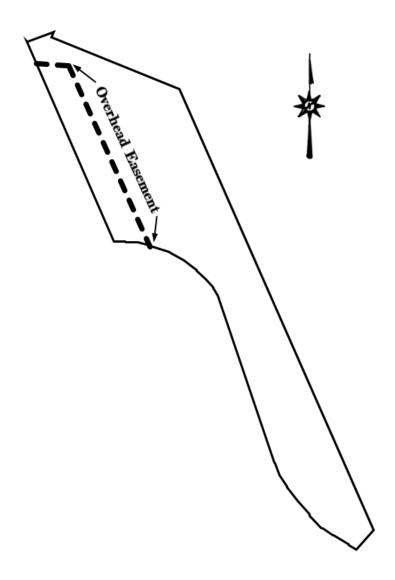
NOTE: The centerline of the powerline as constructed is the center line of the easement.
