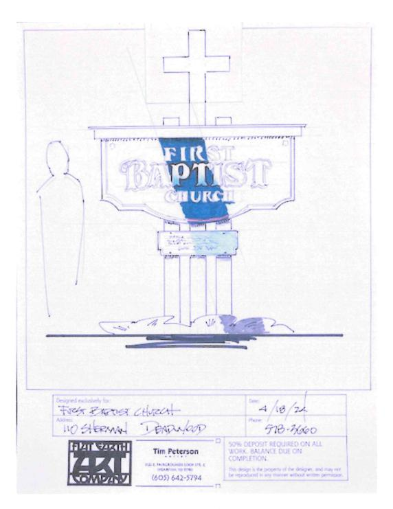
Overall height from grade to top of cross is 9.5 feet. Main sign panel is 3'x 6' with lower information panel 14" x 24" approximately See attached for additional specifications
