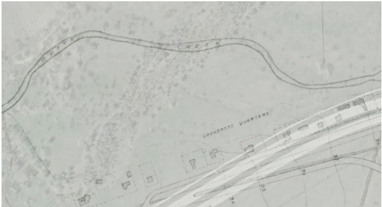
Figure 8. Current bed of Highway 36 (white bands at lower right) overlaid on historic map of Soapsuds Row showing loss of house remains to highway construction.
