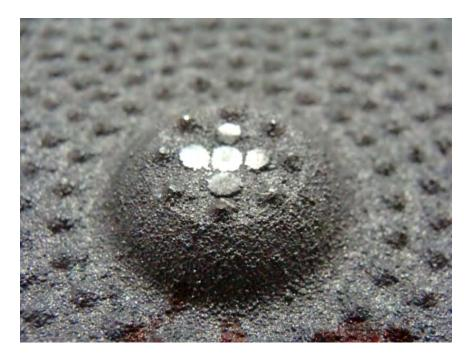
Photo No. 5 - Typical Damage to the Dome After 54 J Impact at Ambient Temperature
