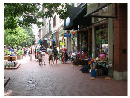
Figure 3. The running bond shown in this image is an example of one way to distinguish the original curb line. Here, the original sidewalk curb line is distinguished along a street that is now a pedestrian mall. This same concept could be applied in Deadwood to distinguish the bumpout from the sidewalk.
