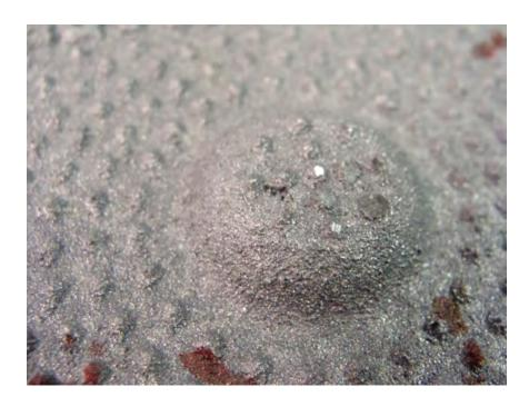
Photo No. 4 – Typical Damage to the Dome After 27 J Impact at Ambient Temperature
