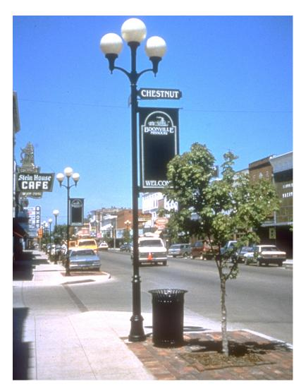
Figure 1. Boonville, MO utilized bumpouts in their historic downtown, which accommodated ramps and globe lights. The bumpout provides additional space to protect the globe lights from any passing vehicles.
