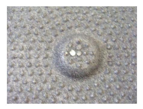
Photo No. 6 - Typical Damage to the Dome After 27 J Impact at -4° C Temperature
