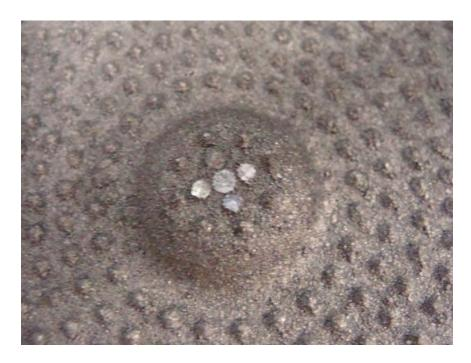
Photo No. 7 - Typical Damage to the Dome After 54 J Impact at -4° C Temperature
