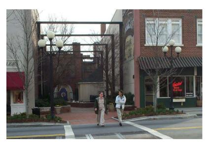
Figure 2. The mid-block bumpout seen in this image protects the globe lights from interference by trucks or other vehicles.
