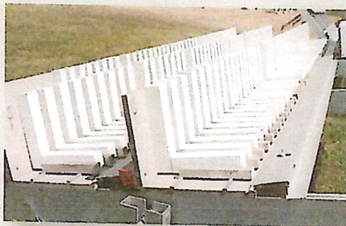
“L-Joint” visual appearance environmental test
