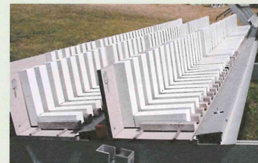
"L-Joint" visual appearance environmental test
