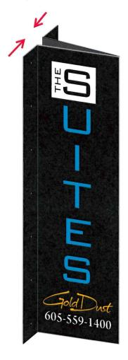
Exploded view. Sign will have 90 degree angle from mounting flanges to projecting portion of sign
