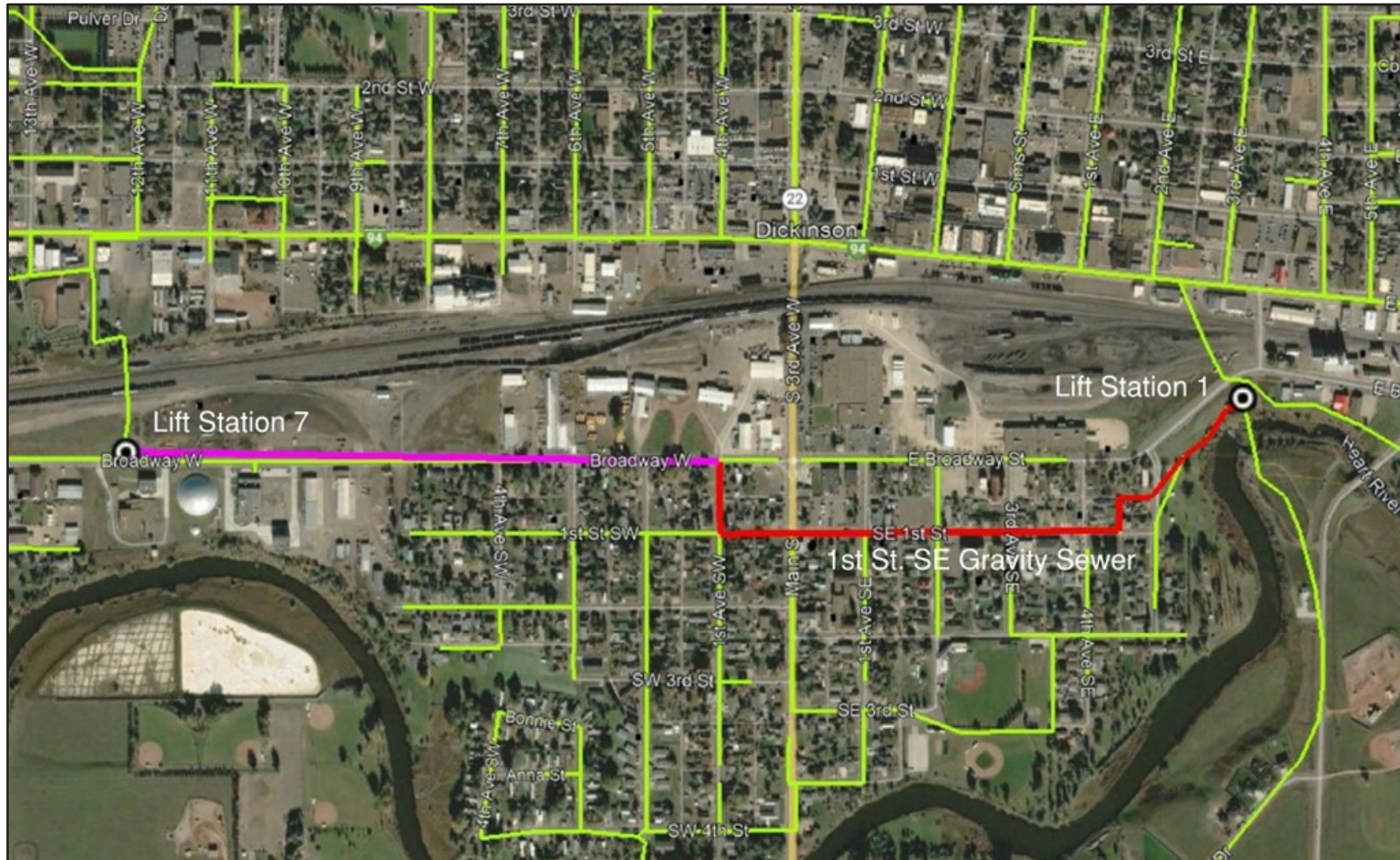
Figure 5 – 1 st Street SE Gravity Sewer
