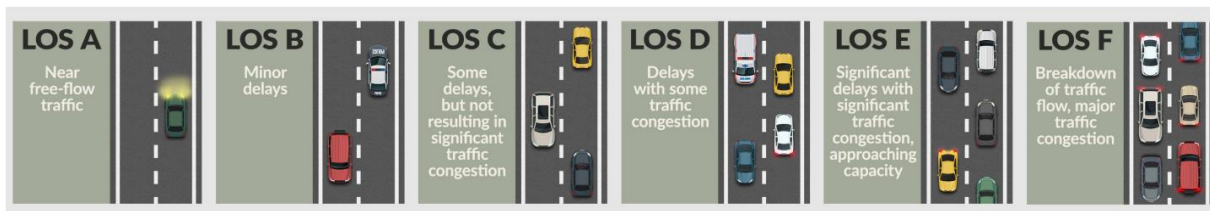
Figure 8-7. LOS Thresholds by Volume-to-Capacity Ratio
