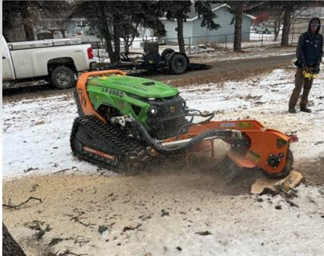
Stump removal using new stump grinder
