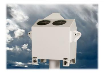
Mesotech's CBME120 ceilometer is a detects cloud height using an eye-safe laser. It uses the Light Detection and Ranging (LIDAR) principle with a low power diode laser. This highly reliable and accurate ceilometer has a detection range up to 40,000 feet (12,000 m).
