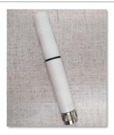
The Mesotech Temperature and Humidity Probe can be used in a wide variety of environments and is excellent for use in automatic meteorological stations. It interfaces easily with data loggers and recorders, is simple to service, and features EMI/RFI protection.
