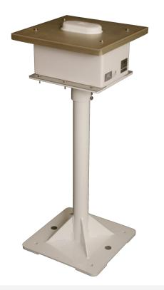
Mesotech's thunderstorm and lightning sensor detects electrical discharges associated with lightning within a 200 nautical mile radius of the system with a <2% false detection rate. This passive lightning detection sensor uses a receiving antenna to "listen" for electromagnetic signals.
