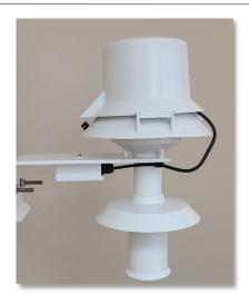
Mesotech's Motor Aspirated Radiation Shield (MARS) provides forced aspiration of a temperature sensor to increase its measurement accuracy in an outdoor environment. Unique in its small size and exceptional performance, this MARS reduces radiation errors to less than 0.2°C RMS with the shield exposed to solar radiation of 1000 W/m<sup>2</sup>.
