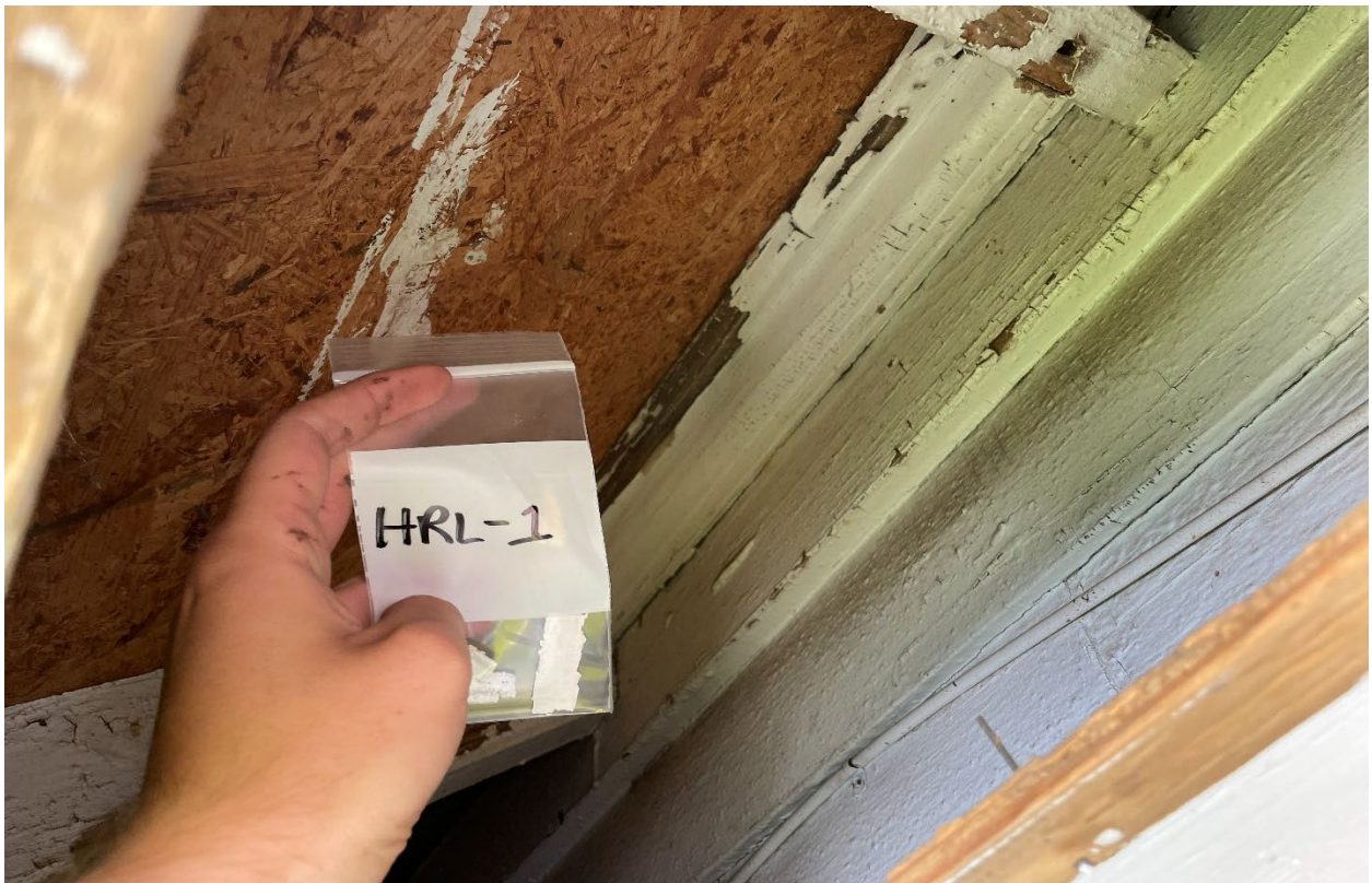
Plate 8: Laboratory analyses detected 5.2% lead within the white paint-like coating within sample HRL-1 collected from the exterior of the structure.
