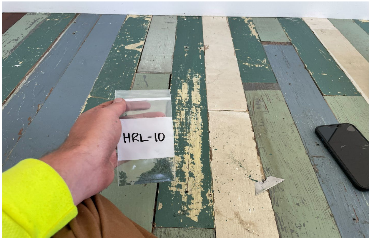
Plate 14: Laboratory analyses detected 0.88% lead within the dark green floor paint within sample HRL-10 collected from the interior of the structure.
