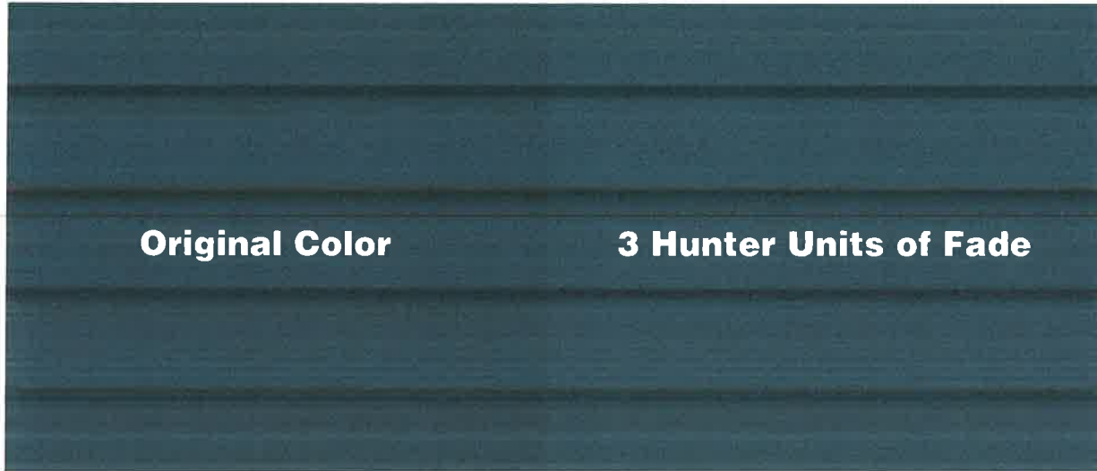
The image is a representation of approximately 3 Hunter Units of fade. Actual fade varies from house to house and is dependent on exposure to weather conditions.
